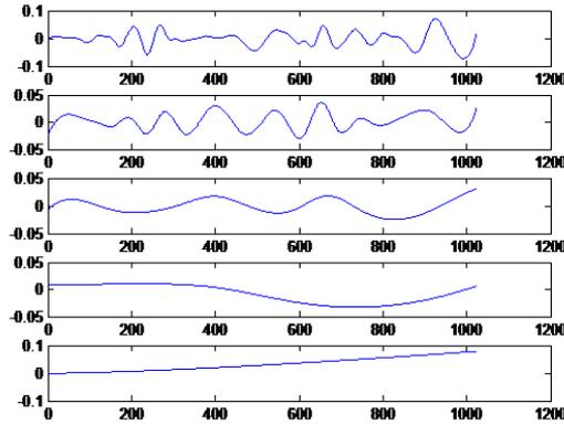
Fig. 2. Eemd decomposition of the outer ring fault signal
